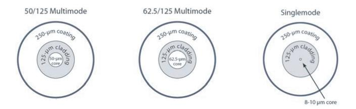
The basic rule of thumb is that the smaller the core diameter, the higher the fiber's bandwidth and the lower the attenuation (loss in dB per kilometer). The fiber's attenuation and bandwidth are also dependent on wavelength. The table below illustrates the approximate attenuation of both multimode & singlemode fibers.
